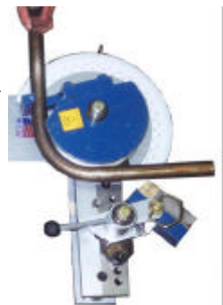
Left—The M-150-S can produce a 180 degree bend in approximately 23 seconds.
